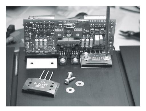
Lay the heatsink down and place the (orange) Kapton sheets over each pair of mounting holes for the output devices. No grease is called for!
