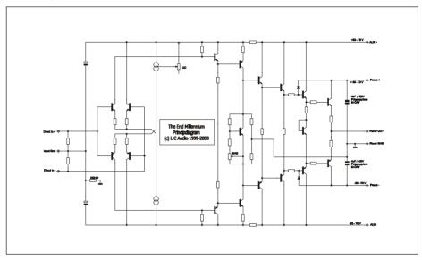
The principle schematic shows how simple the fundamental circuit of Millennium really is. There are no feedback loops (100% non-feedback), there are no capacitors or other sound depriving components near the signal path. The frequency responce is linear from DC to extreme hights: 500.000 Hz. This is probably the fastest amplifier You ever heard! Any part of the music from the deepest bass to the teeniest transient is reproduced with ease by the Millennium!
