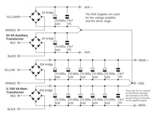
The Power supply unit consist of 120.000 American made MicroFarads, and provides all the stability and musclepower needed to drive even critical speaker loads. The brand ChemiCon is formerly known as Sprague.
