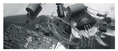
Start by mounting the lowprofile components, like resistors and trimmers. Follow the printed values on the PCB itself, and compare with the color codes printed on the previous page. If You are sure everything is mounted correctly, solder it down. After this fit the capacitors, first the smaller ones and then the larger ones. Solder.
